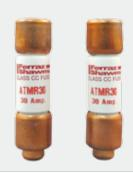
Amp-Trap® ATMR fuses, in the Class CC family, are the smallest dimension 600VAC/DC fuses suitable for branch circuit protection. The ATMR is a popular choice for economical protection of control circuits and control circuit transformers where available short circuit currents exceed 10,000 amperes. ATMR's rejection dimensions prevent substitution by lesser rated fuses. These fast acting fuses give currentlimiting protection to general circuits.
